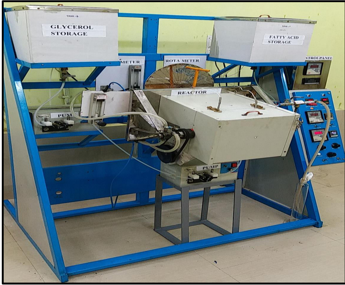
Fig.12. Photograph of electromagnetically radiated rotating continuous flow packed bed reactor.
