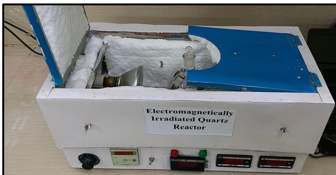
Fig.1. Photograph of infrared radiated rotating Batch Reactor
